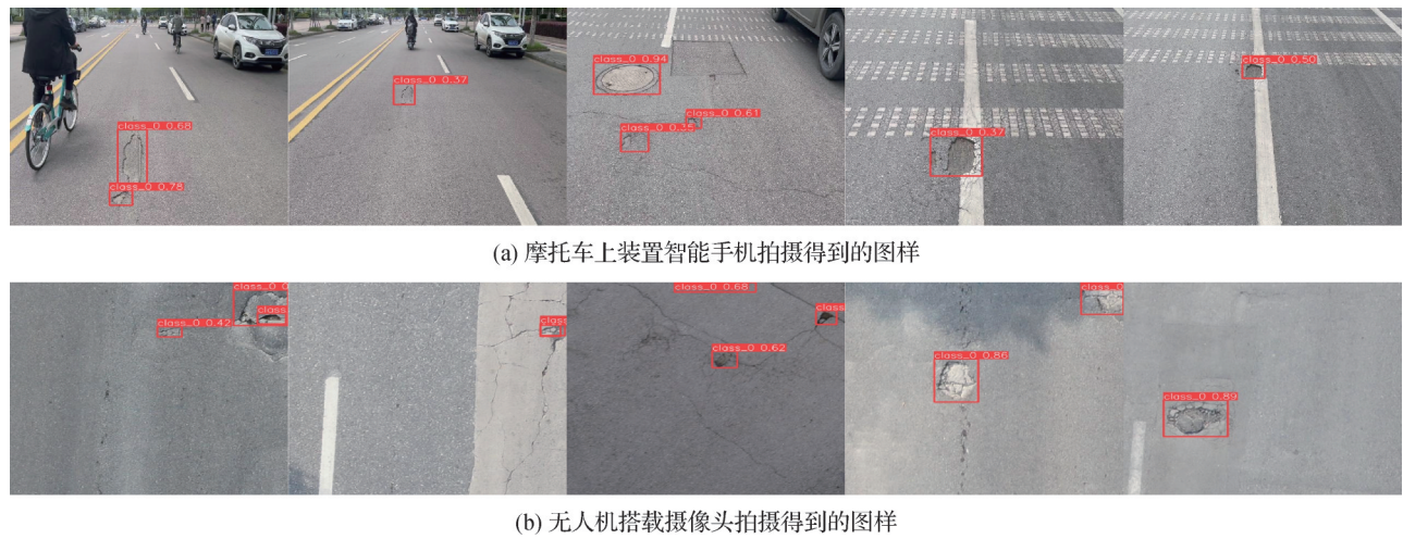
图 16 模拟实际场景的路面坑洞检测效果 Fig. 16 The pavement pothole detection effect of simulating the actual scene ( (a) images captured by a smartphone attached to a motorcycle; (b) images captured by a camera mounted on a drone )
