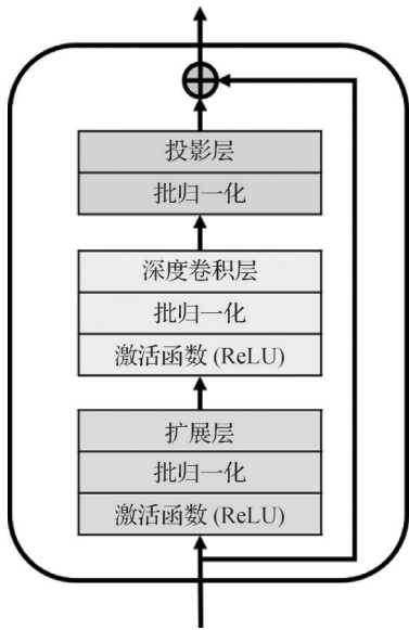
图 3 倒残差块结构 Fig. 3 Structure of inverted residual block
