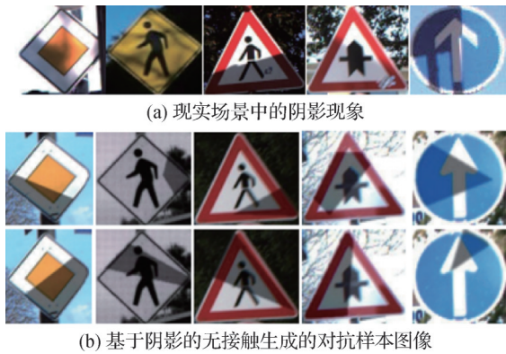
图 31 基于阴影的无接触对抗攻击(Zhong 等,2022) Fig. 31 Shadow based contactless adversarial attack (Zhong et al. , 2022) ((a) shadow phenomenon in real scenes; (b) adversarial sample images generated based on shadow casting)
