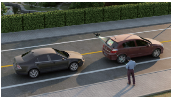
图 32 对抗图案投影至车辆后侧窗口的应用示意图 (Wen 等,2024) Fig. 32 Application example of projecting adversarial patterns onto the rear window of a vehicle (Wen et al. , 2024)
