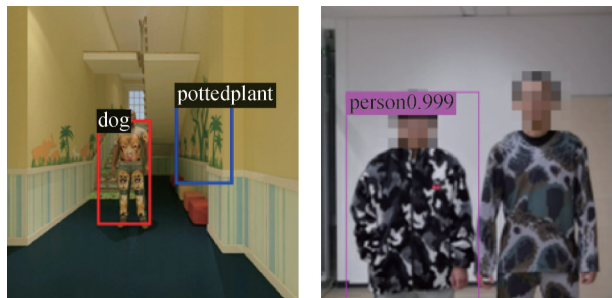
图35 针对行人检测的3D渲染物理对抗攻击 (Huang等,2020;Hu等,2023b) Fig. 35 3D rendering-based physical adversarial attack against pedestrian detection (Huang et al. , 2020; Hu et al. , 2023b)
