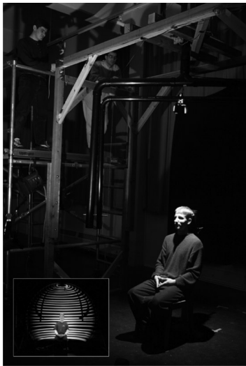
图 5 Light Stage 人脸捕获设备(Debevec 等,2000) Fig. 5 Light Stage facial capture system (Debevec et al. , 2000)
