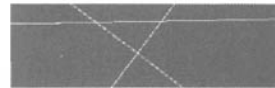
图 6 Hough 变换后的 V 型坡口图样 Fig. 6 The figure of V-groove after hough transform
