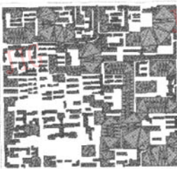
图 3 对建筑物构建 TIN 网 Fig.3 Building TIN net to city buildings
