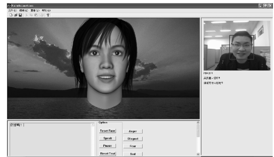
图 13 虚拟人通过分析交互者的表情来进行情感交互 Fig. 13 Virtual human will do emotion interaction by analyzing human’s facial expression
