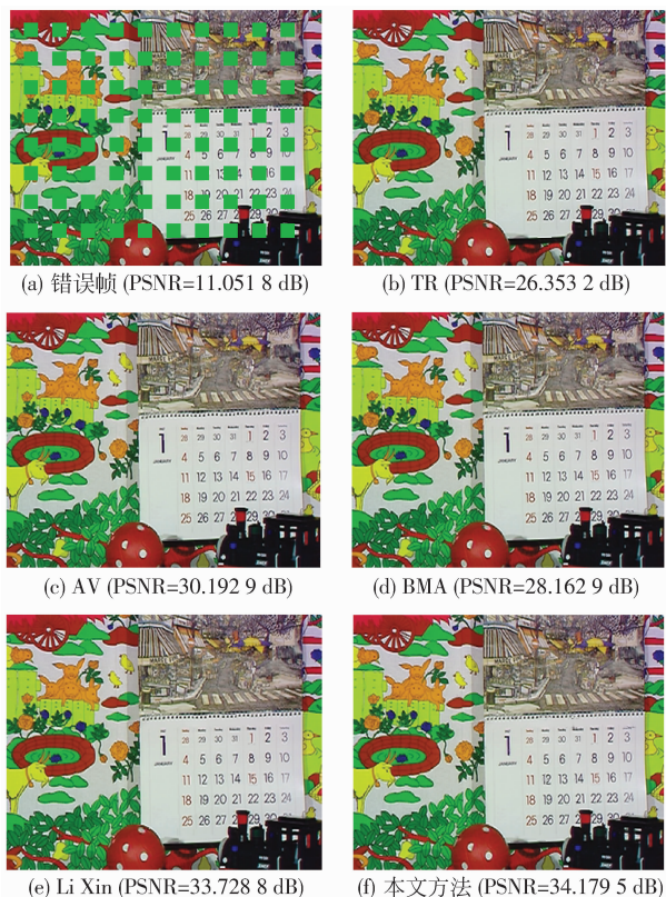
图 3 mobile 序列第 29 帧独立丢失块几种方法性能比较 Fig.3 The comparison of the result for isolated block loss from different methods of the 29th frame in mobile
