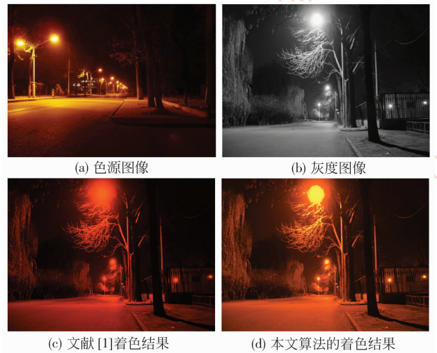
图 7 实验结果比较 Fig. 7 The contrast of colorization results between different methods
