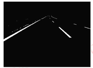
图 5 消隐线上方置黑 Fig.5 Set the area above the elapse line as the black zone
