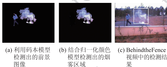
图2 利用改进的颜色模型进行烟雾检测的实验结果 Fig. 2 The result of smoke detection using the improved color model
