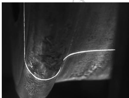
图1 线结构光在轮对上的投影 Fig.1 Structured light projection on wheel set
