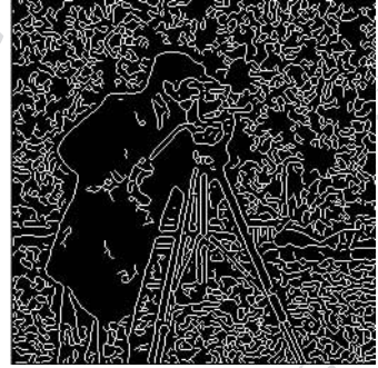
图 11 含噪 Canny 默认阈值下的检测结果 Fig. 11 The result of Canny operator with noise when the threshold is default
