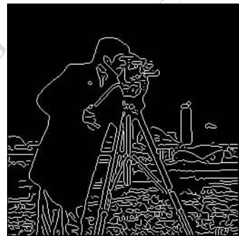
图7 默认阈值下的 Canny 检测结果 Fig.7 The result of Canny operator with default threshold
