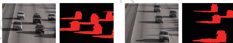
图8 含有大量阴影时的运动检测结果(Highway I) Fig. 8 Moving pixel detection with large shadows (Highway I)
