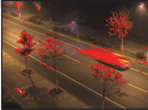
Dynamic target detection and tracking based on fast computation using sparse optical flow (P1593)
