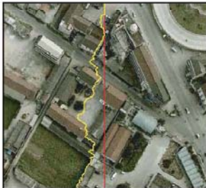
Finding an optimal seam-line through the shortest distance in the neighborhood(P227)
