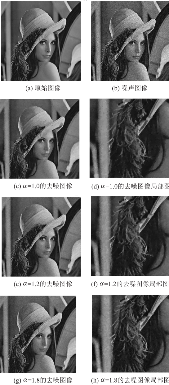
图 3 典型阶次下去噪效果及其局部效果的比较 Fig. 3 Comparison of denoised results and their local enlargements under classical orders
