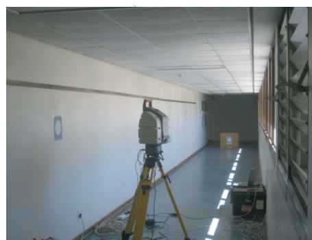
Fig. 2 Experimental plane and flat target
