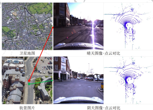
图3 不同光照条件下同一地点相机与LiDAR观测结果对比 Fig. 3 Comparison between image-based and LiDAR-based localization
